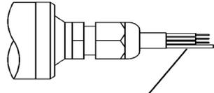
For cable version: Vented cable with capillary
